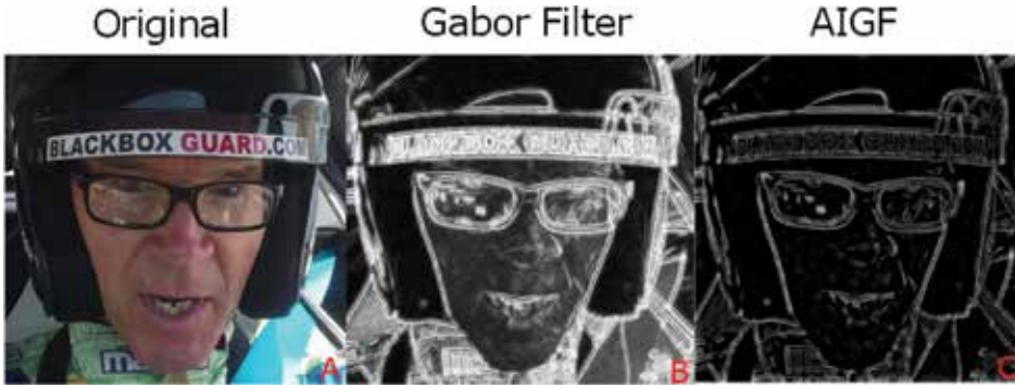
Figure 2. (a) Original frame, (b) result of Gabor energy filter (Eq. (15) with \alpha = 0 ), and (c) result of Anisotropic Gabor Energy Filtering.
