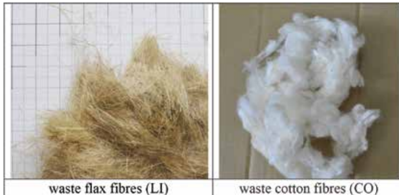
Figure 1. Photographs of the waste natural fibres reinforcement.
