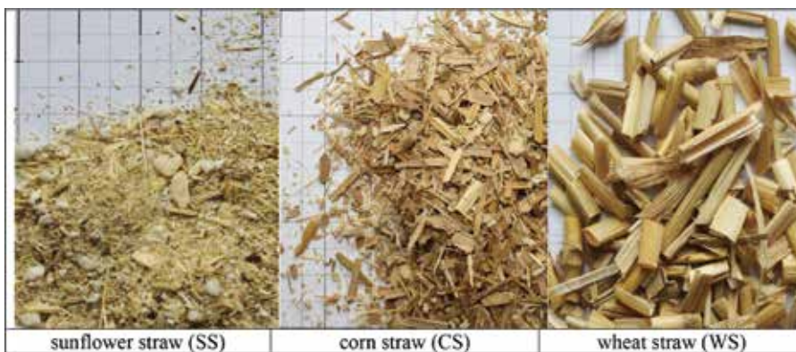
Figure 2. Photographs of the straw reinforcement.
