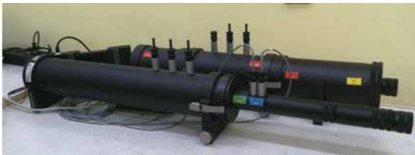
Figure 6. The Kundt device for acoustic measurements.
