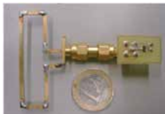
Figure 15. Folded dipole implementation at 300MHz [64].
