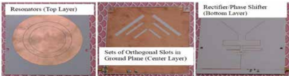
Figure 12. Slot-coupled multiresonator (tri-band).
