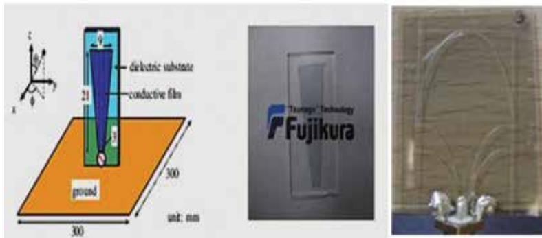
Figure 8. Transparent radiator of the monopole antenna.
