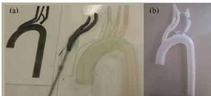
Figure 2. (a) Fitting the hybrid bypass mold to the real size model according to surgery specifications and (b) the resulted model.
