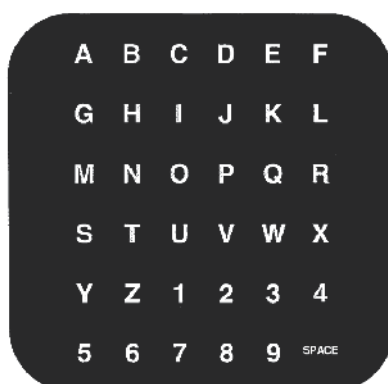
Fig. 3. The matrix for P300 speller. The stimulus matrix monitored by the subject. Typically, one of the rows or columns of the matrix was intensified every 125 ms (The matrix is proposed first by Donchin and colleagues 1988).
