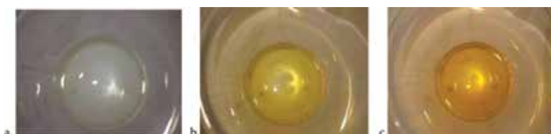
Figure 1. Photographs of PAN/10 wt% AgNO 3 solution: (a) without any treatment; (b) after exposure to xenon-arc lamp for 15 min; (c) after exposure to xenon-arc lamp for 30 min.
