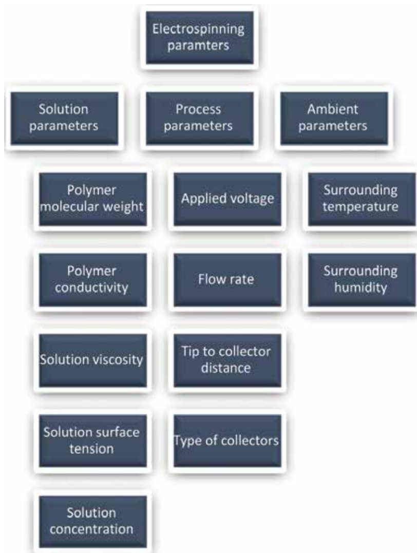
Figure 2. Factors affecting on elctrospinning technique.
