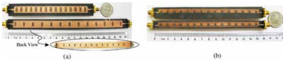
Figure 7. Fabricated LWAs, (a) SIW configuration and (b) HMSIW configuration [7].
