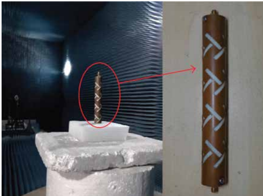
Figure 10. Photograph of the omnidirectional dual CP antenna being tested in the anechoic chamber.
