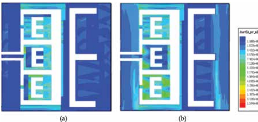
Figure 6. Current density distribution over the antenna at (a) 4.75 GHz and (b) 7 GHz.
