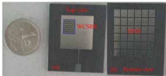
Figure 19. Photograph of the fabricated proposed antenna. (a) Top view; (b) bottom view [30].
