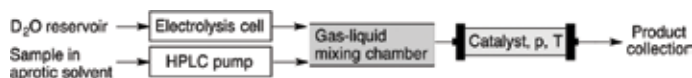
Figure 18. Schematic outline of the continuous flow reactor used to prepare deuterated compounds by Hsieh et al [48].
