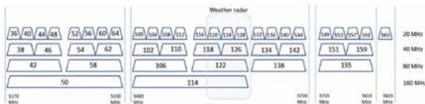
Figure 5. 5 GHz channels for IEEE 802.11.
