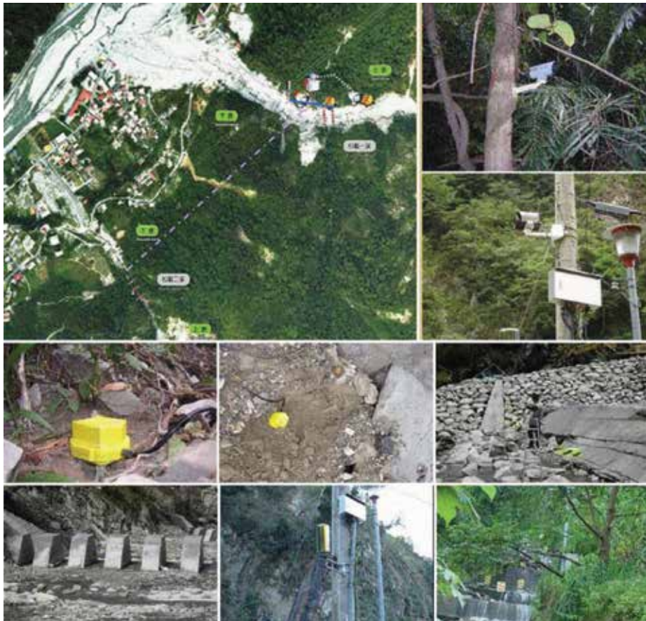
Figure 17. The equipment at the Songhe Debris Flow Monitoring Station includes one rain gauge, two CCD cameras, two geophones and eight wire sensors.
