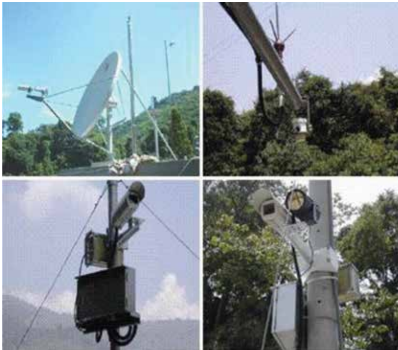
Figure 15. The equipment at the Fengqiu Debris Flow Monitoring Station include one rain gauge, two CCD cameras, two geophones, four wire sensors and one water-level meter.
