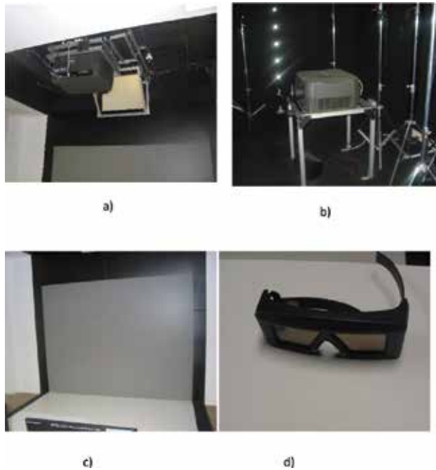
Figure 1. Elements of the virtual reality room. (a) and (b) Projectors, (c) 2 screens in an L shape, and (d) virtual reality glasses.
