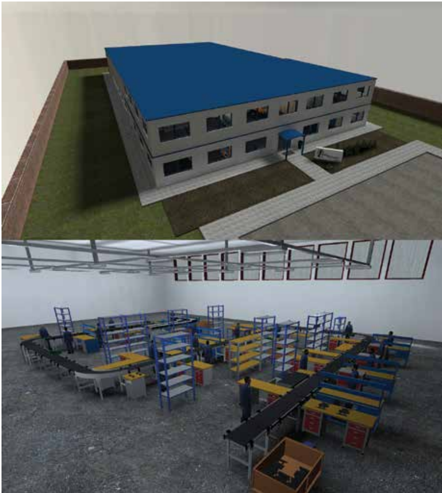
Figure 2. The Half-Life 2 production line validation model. Above is an overall view of the building and parking place. Below is the redesigned production line.
