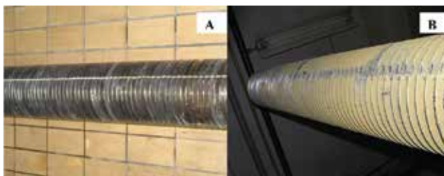
Figure 3. O-shaped rings before (A) and after (B) biofilm formation in HRTB.
