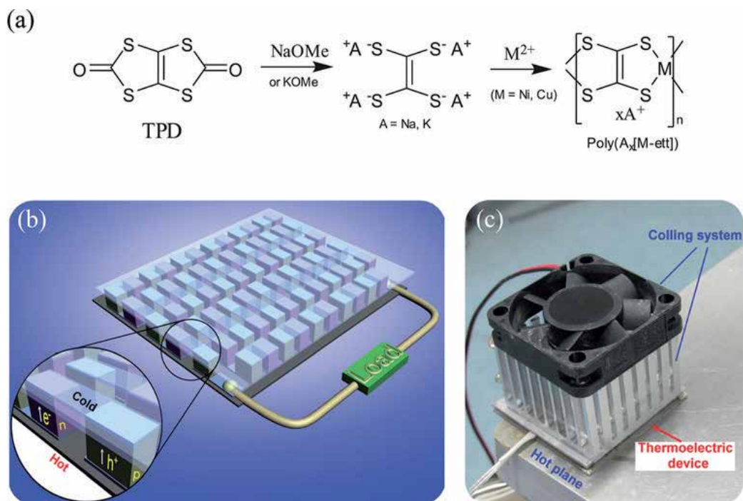
Figure 3. (a) Synthetic route of poly[ A_x[M\text{-ett}]_n ], (b) module structure and (c) photograph of module and measurement system with a hot plane and cooling fan.
