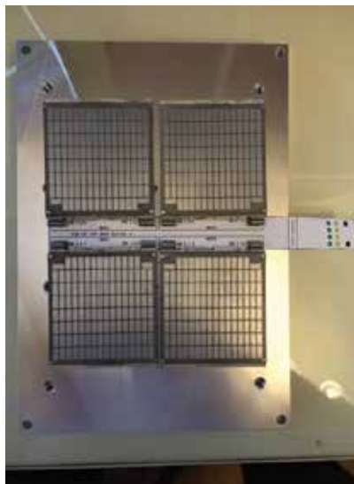
Figure 18. Four Hi-Z-14 modules on a water-cooled plate.
