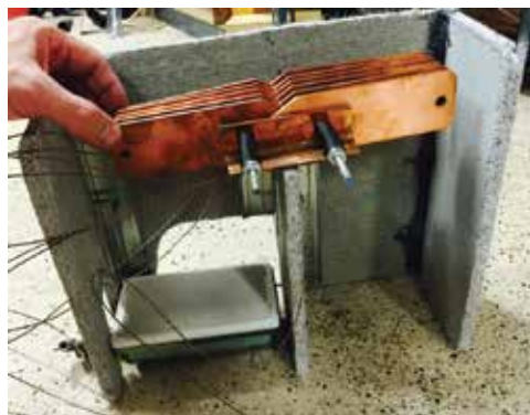
Figure 14. Lateral view of inside of P1 prototype TE generator, left side at the bottom is the infrared burner, combustion gases go upwards; in the centre at top, column structure-heated blades; to the left, cooled blades by ambient air blown upwards (fan is not shown).
