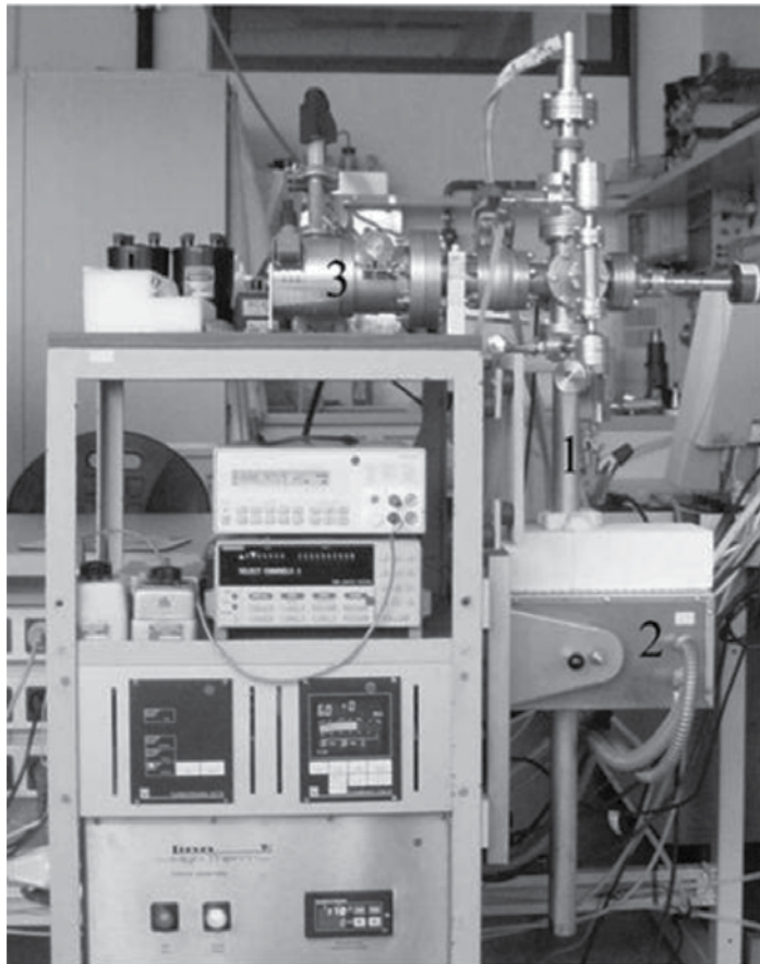
Figure 18. Experimental set-up for thermopower and electrical conductivity measurements at 80–1300 K.
