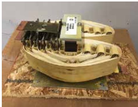
Figure 17. PWM 10 kW transformer dimensions 250 × 190 × 140 mm high.
