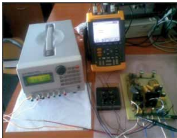
Figure 23. The microactuator with magnetic nanofluid during testing [68].
