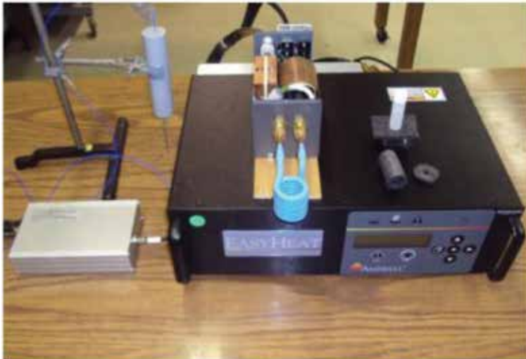
Figure 9. Ambrell Easy Heat System with coil, sample holder, insulating cotton padding, and OPTOCON fiber optic thermometer.
