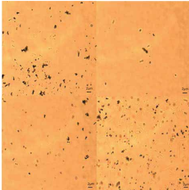
Figure 4. Microscopic 100× images showing the Ag NPs coverage of bacteria ( E. coli ) when using the in situ synthesis approach (Bacteria@ Ag NPs).
