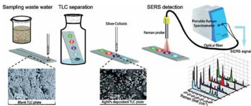
Figure 4. Schematic illustration of TLC-SERS for on-site detection of substitute aromatic pollutants in waste water. Reproduced with the permission from Ref. [77].
