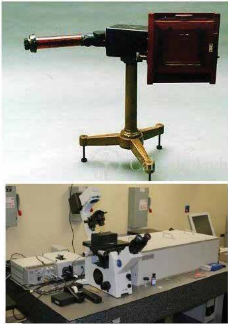
Figure 2. The development of Raman instrumentation from the Raman spectrometer of C. V. Raman to the latest sophisticated Horiba-Jobin model of the micro-Raman system.
