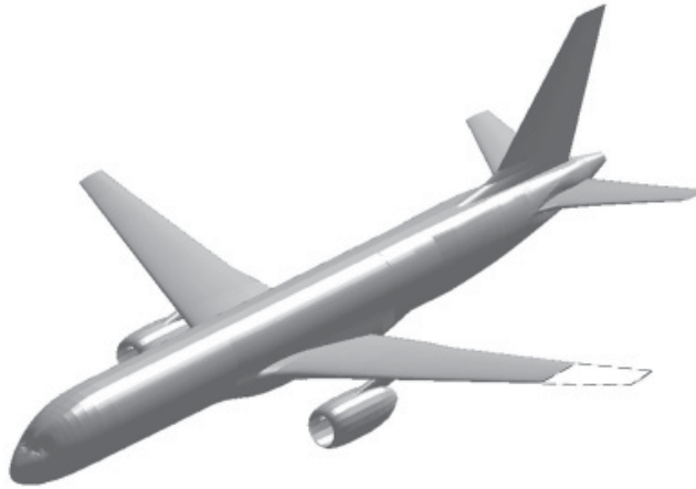
Fig. 2. Left Wing Damaged Generic Transport Model
