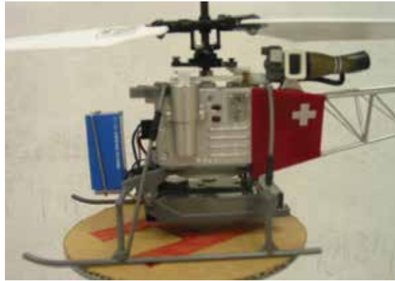
Fig. 3. RC helicopter equipped with a micro wireless camera
