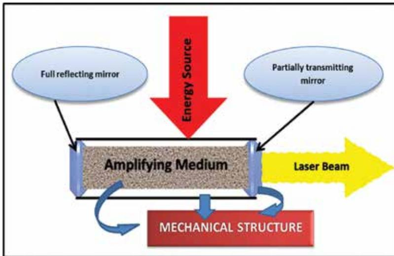
**Figure 3.** Simplified schematic of laser basic components.
