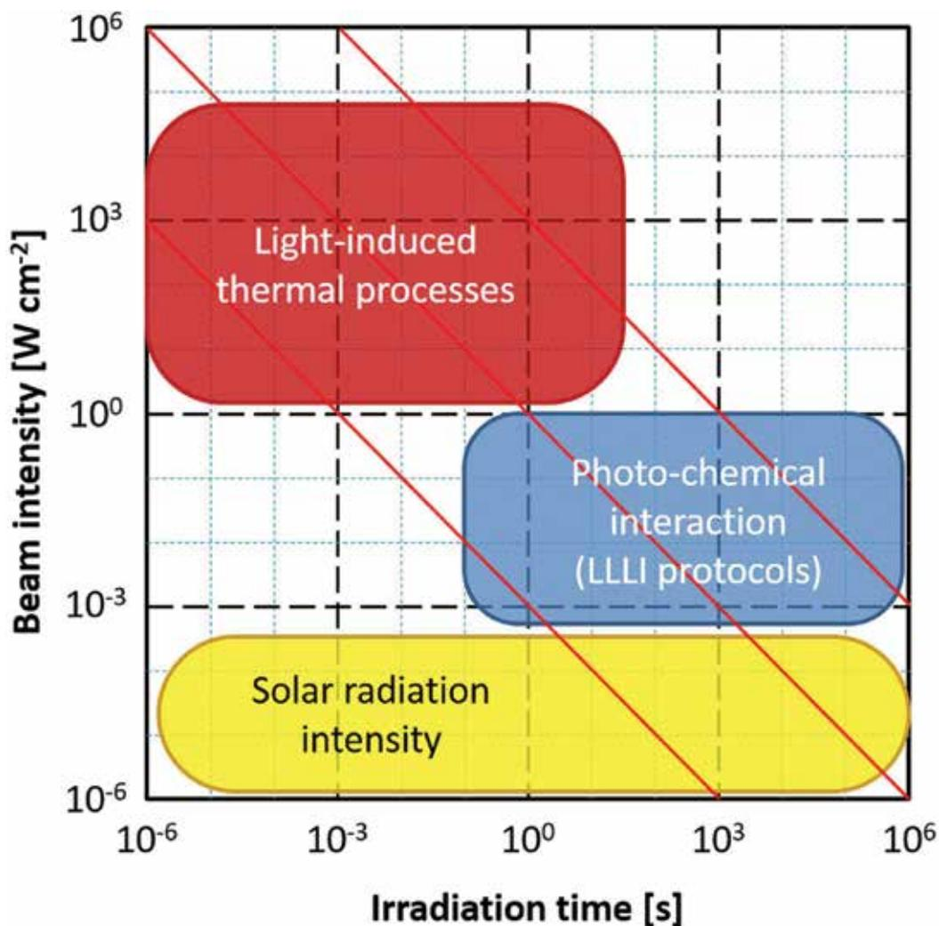
Figure 4. Log-log chart describing the interactions produced as a function of the beam intensity and of the irradiation time.
