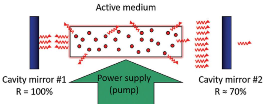
Figure 3. Example of the generation of laser beam into a cavity.
