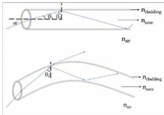
**Figure 3.** Multiple reflections in a bent optical fiber.
