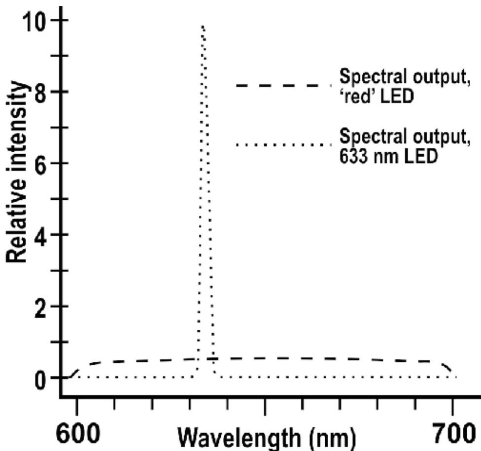
**Figure 1.** Difference in spectral distribution and relative output power (photon intensity) between an old-generation broad bandwidth red light-emitting diode (LED) and the new generation type, emitting in the example shown at  $633 \pm 5$  nm. With the new generation LEDs, even though they are non-coherent, more than 90% of the photons are emitted at the rated wavelength with a very narrow bandwidth, conferring quasimonochromaticity on the beam.
