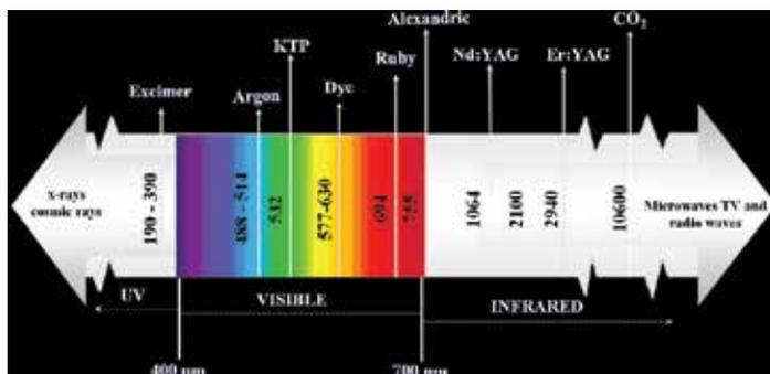
**Figure 1.** IPL is situated in the visible light and infrared radiation of the electromagnetic spectrum (reprinted with permission of Lumenis company, Yokneam, Israel).
