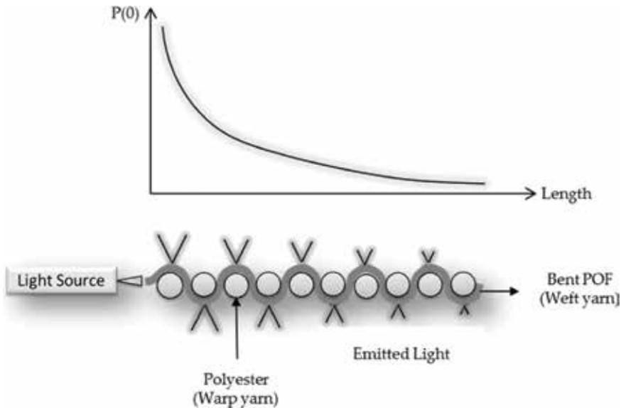
**Figure 5.** Bending loss in a POF inserted in a woven fabric.
