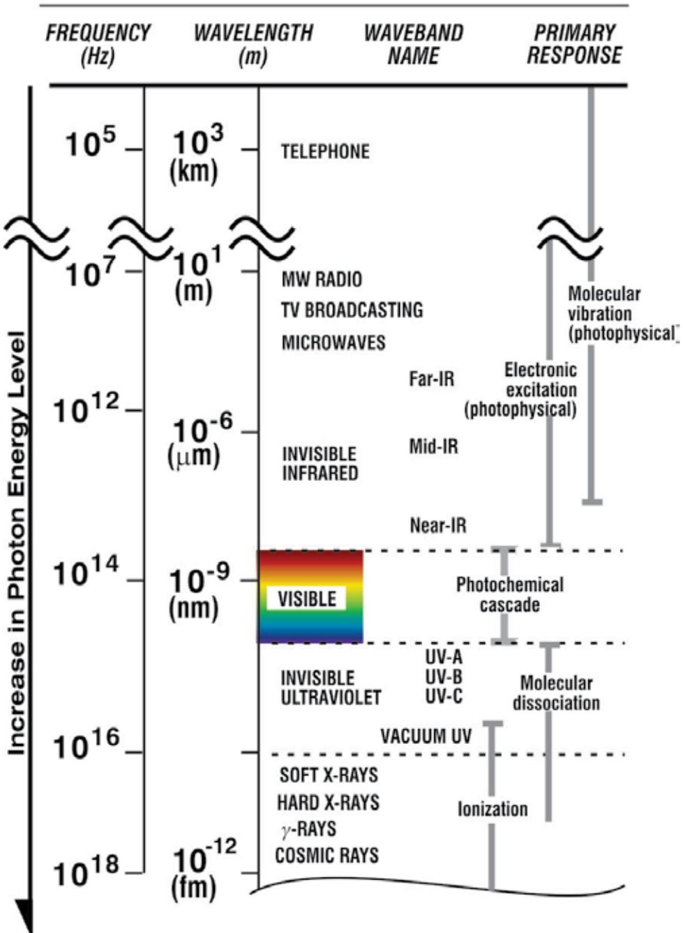
**Figure 7.** The electromagnetic spectrum (EM) covers a vast range of energy radiation types extending from the shortest cosmic waves (wavelengths measured in femtometers [fm] or shorter), through ultraviolet and visible radiation (nm), infrared radiation ( $\mu$ m) to the broadcasting waveband (m) and even mains current and wired telephone transmission (km).
