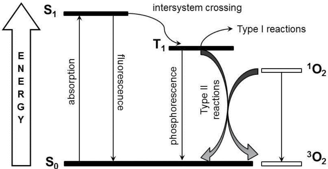
**Figure 1.** Simplified Jablonski diagram for energy transition between states and from photosensitizers in excited states to molecular oxygen, producing singlet oxygen and other reactive species.
