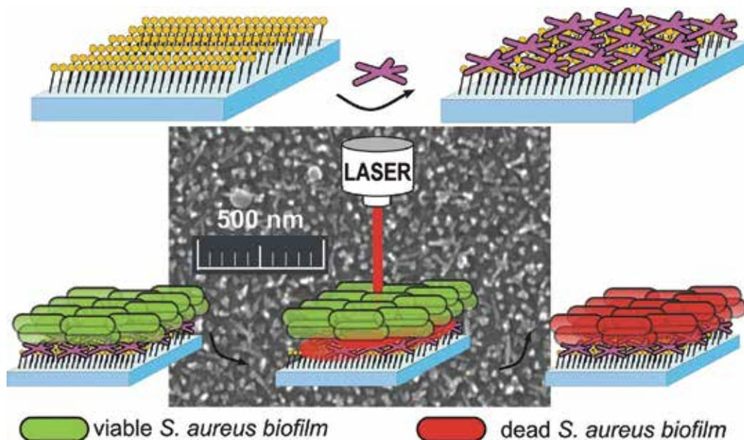
**Figure 5.** Monolayers of gold nanostars (GNS) grafted on mercaptopropyltrimethoxysilane-coated glass slides for aPDT application.
