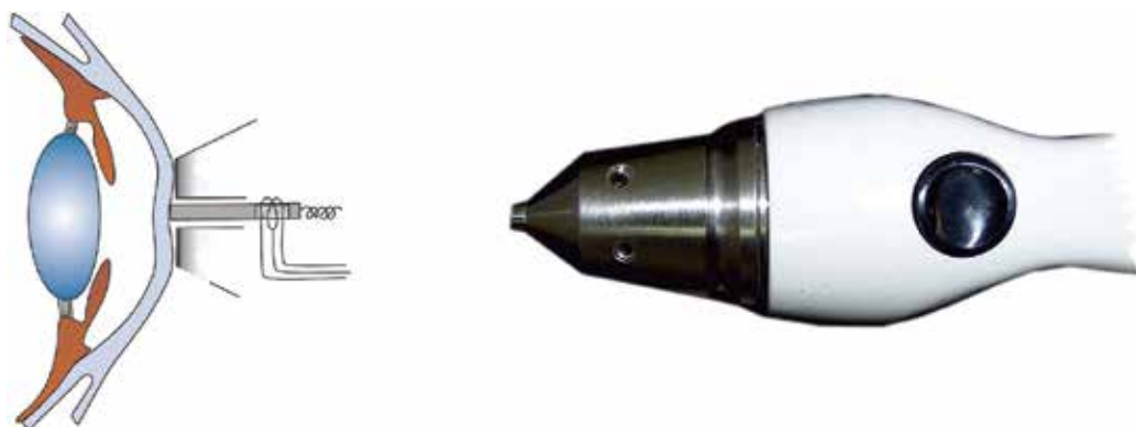
Figure 5. A schematic representation describing the working principle of Tono-Pen.
