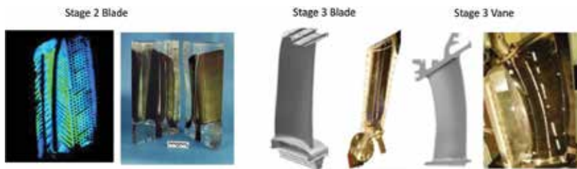
Figure 35. Perspex model testing of gas turbine blades and vanes [2].
