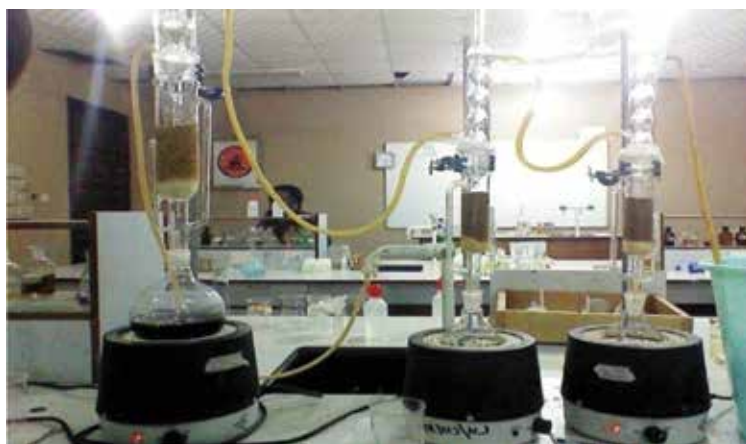
Figure 3. Three soxhlet apparatus on heating mantles during the hot extraction of the phytochemicals in water melon rind (Source: Authors).
