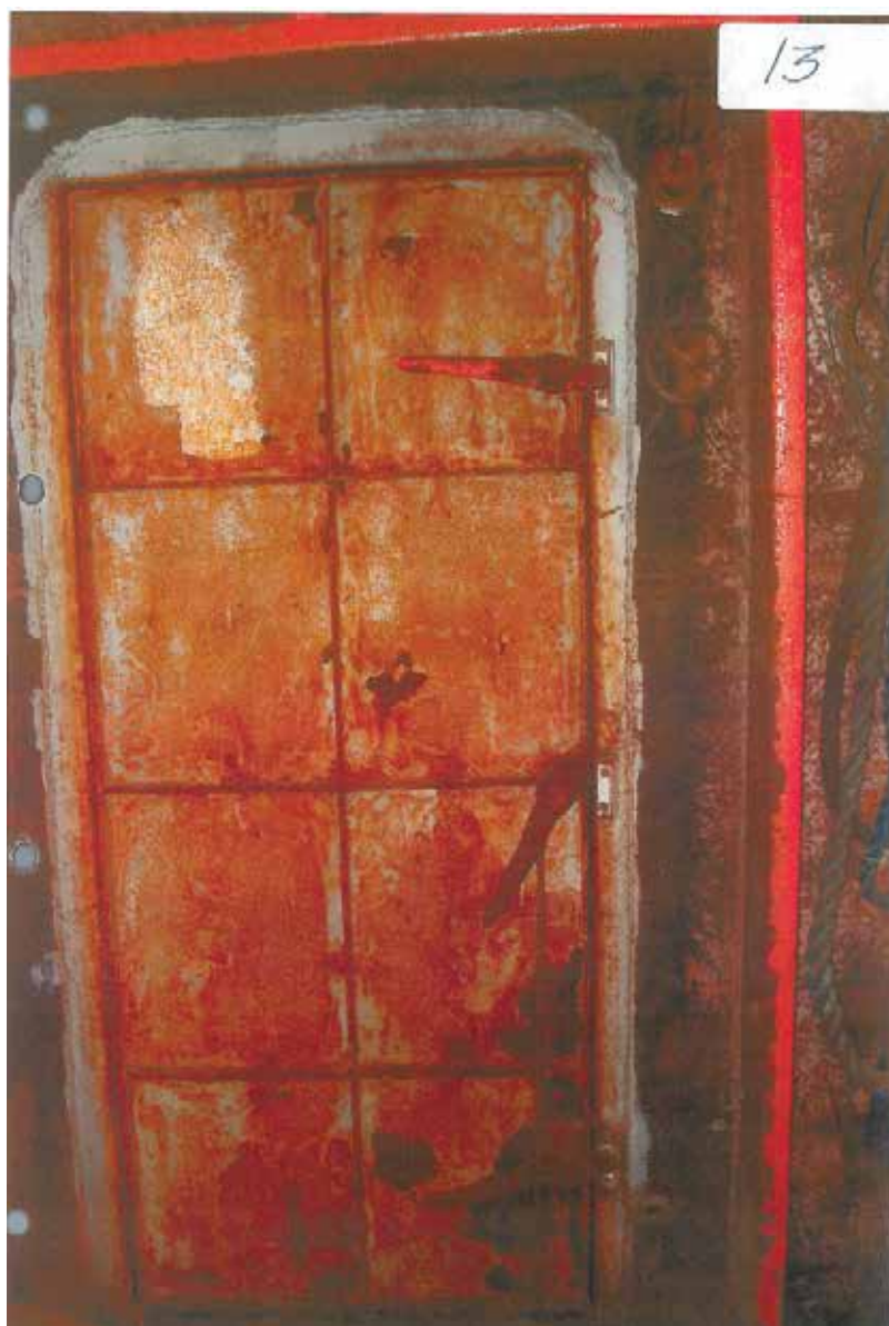
Figure 1. The door in the forepeak compartment, which led the front cargo hold. The door had three closing hinges but only two were engaged. Gasses travelled from the cargo hold to the forepeak through a crevice where the third hinge was not engaged. (AMIRANTE). Source: Police photo file #13 [8].
