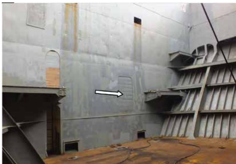
Figure 3. An opening in the front cargo hold allowed easy access to the lashing equipment room. When carrying bulk cargo, the opening was closed with planks of wood inserted into guide bars (CORINA). Source: [16].
