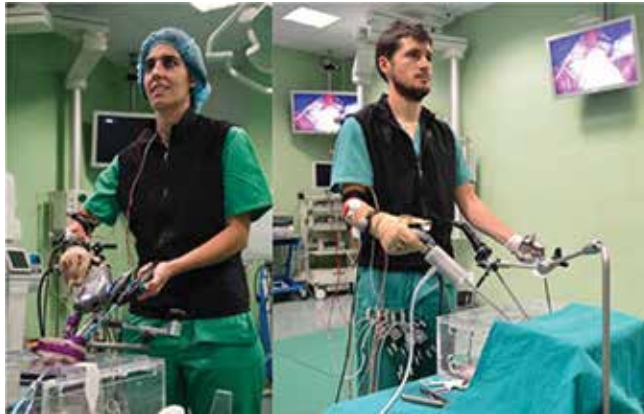
Figure 8. Setup for the ergonomic study in the training environment using (left) the Kymerax™ and (right) the DEX™ handheld robotic instruments.
