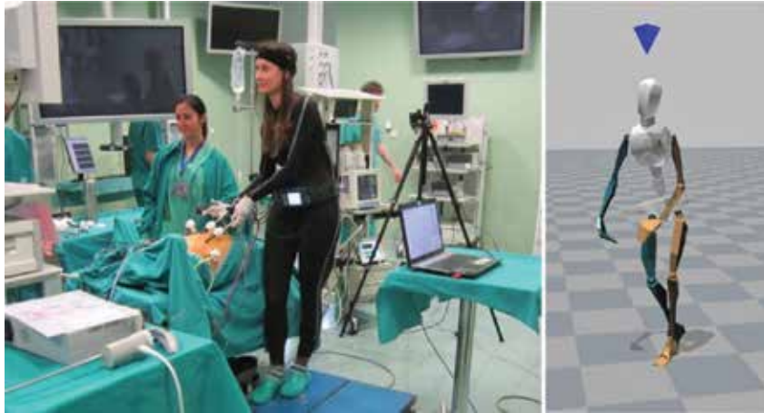
Figure 2. Motion tracking system based on inertial sensors embedded in an elastic suit ( left ). A biomechanical model of the subject is created in real time ( right ).
