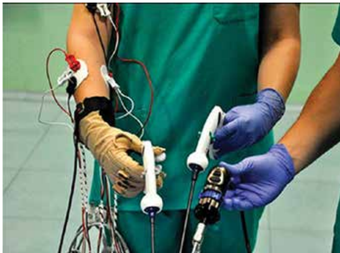
Figure 7. EMG and data glove data acquisition during the performance of hands-on simulator tasks using a LESS approach.
