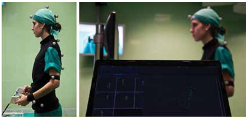
Figure 1. Motion tracking system based on retro-reflective markers. Artificial markers are placed on the targeted segments of the surgeon's body ( left ). A software application computes the kinematics variables during the task execution ( right ).
