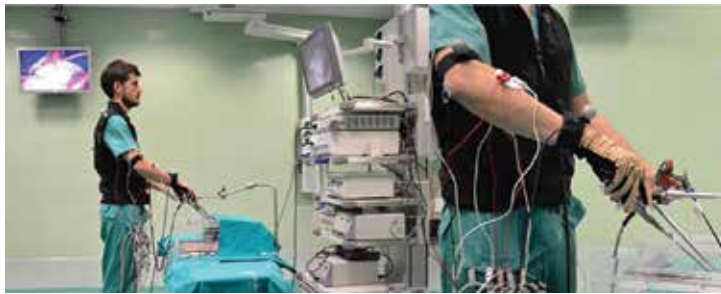
Figure 6. EMG and data glove data acquisition during the performance of laparoscopic tasks on simulator.
