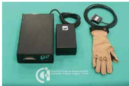
Figure 4. Motion capture data glove CyberGlove® (CyberGlove Systems, San José, CA, USA). This device consists of a series of conductive sensors with resistance flows sensitive to flexion variations.
