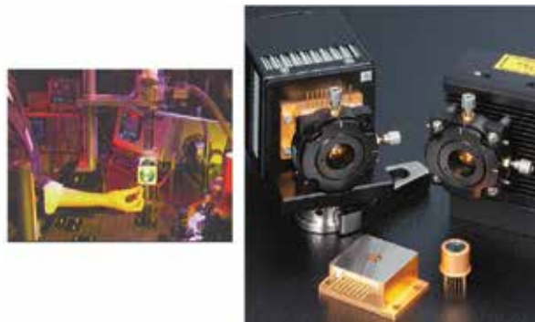
Figure 2. Left: the invisible beam from a high-power quantum cascade laser lights a match in its path. The laser is 2.25 mm long and 17 \mu\text{m} wide, being placed in a cryostat at liquid-nitrogen temperature and emits an optical power in excess of 200 mW from each facet at a wavelength of 8.0 \mu\text{m} . Similar devices emit up to 600 mW at room temperature in pulsed mode. Right: front: mid-IR lasers (4–10 \mu\text{m} ) for trace-gas analysis and IR molecular spectroscopy in the front; back: set-up examples.
