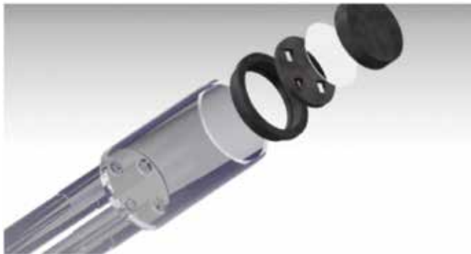
Figure 15. Upper part of quartz reactor with sample holder and substrate.
