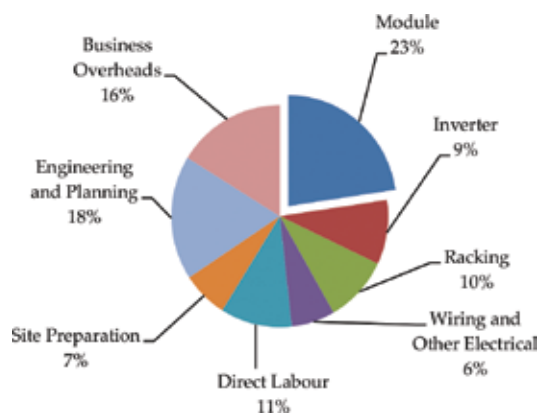
Figure 3. Breakdown of costs for PV systems. Source: Chung et al. [9] and IRENA Secretariat [10].
