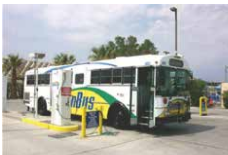
Figure 11. A 40-foot-long transit bus at SunLine Transit Agency with HCNG dispenser [59].
