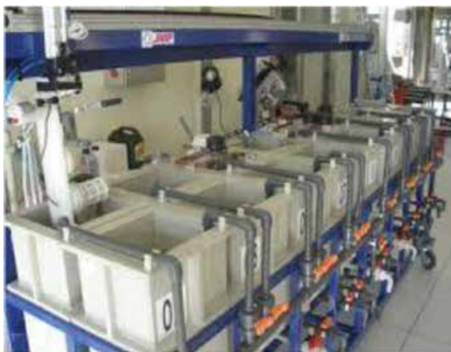
Figure 4. A chrome plating pilot plant part of the IONMET consortium activities [80].
