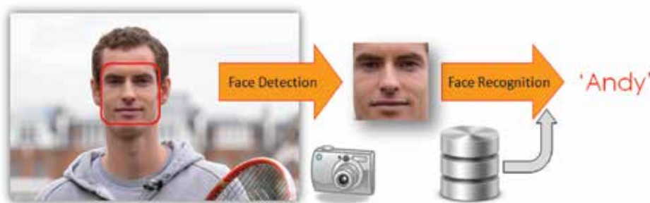
Figure 1. Overview of the face detection and recognition processes.
