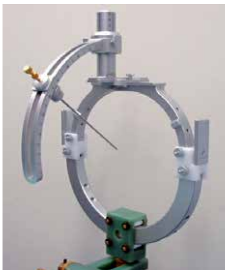
Fig. 3. Head-holder coil integrated with modified Komai stereotactic frame for stereotactically guided surgical procedures under the control of intraoperative MRI.
