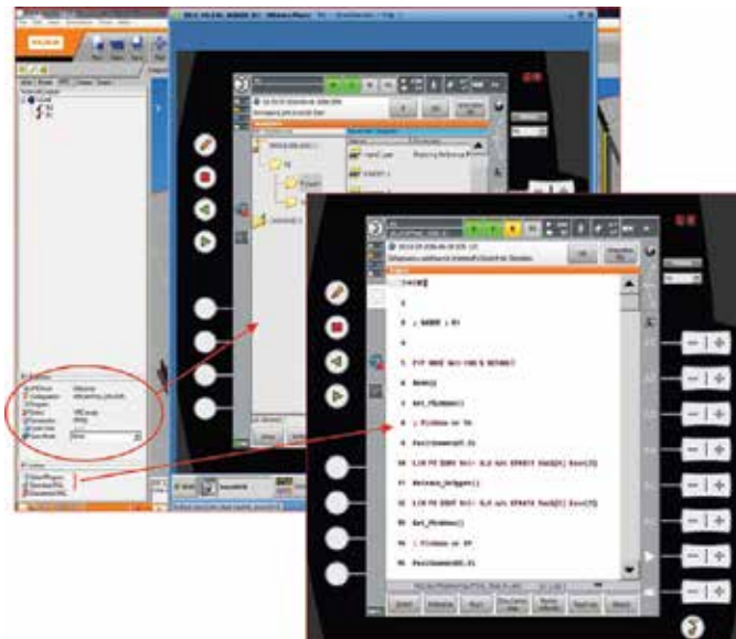
Figure 12. 'Cutting_head_R1' utility programme for the robot positioning the pickboxes generated in KUKA.SimPro environment transferred to the virtual operating system of KUKA.OfficeLite robot.
