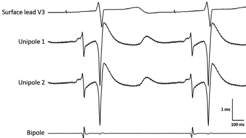
Figure 3. Relationship between different types of electrograms: The top-most plot is the surface lead which illustrates the QRS complex. The next two signals are two closely spaced unipoles; the far-field ventricular activations can be clearly seen in them. The last signal is the resultant bipole of the two unipoles in the figure. It can be clearly seen that the ventricular activations gets canceled giving rise to atrial activations alone. Also, the baseline noise present in unipoles is removed in the bipole signal.
