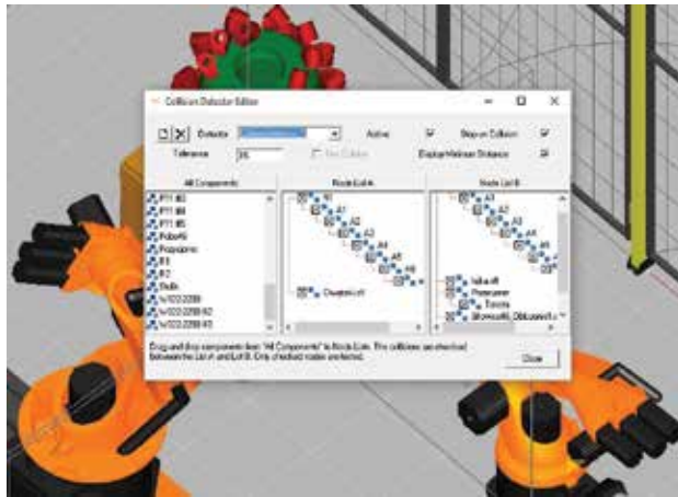
Figure 11. Collision detection module in KUKA.SimPro environment.
