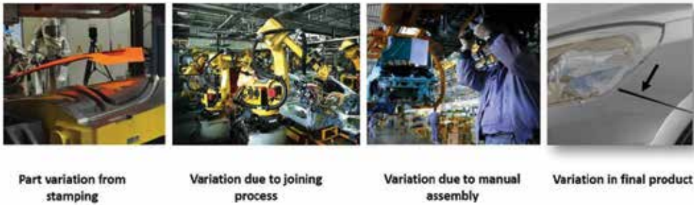
Figure 1. A nonparallel split line, caused by variation due to the stamping, joining and assembly processes.
