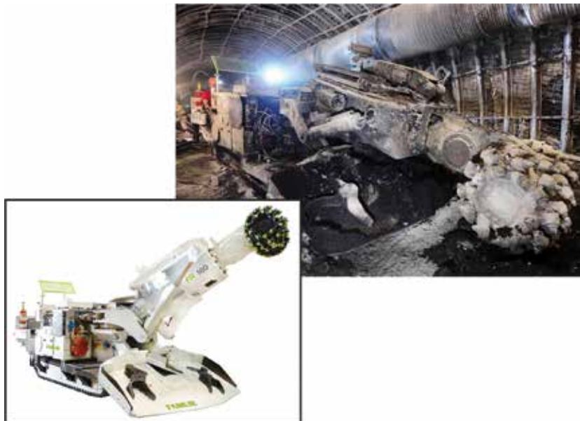
Figure 1. Boom-type FR 160 roadheader designed for drilling dog headings in underground mines and tunnels in civil engineering [6].
