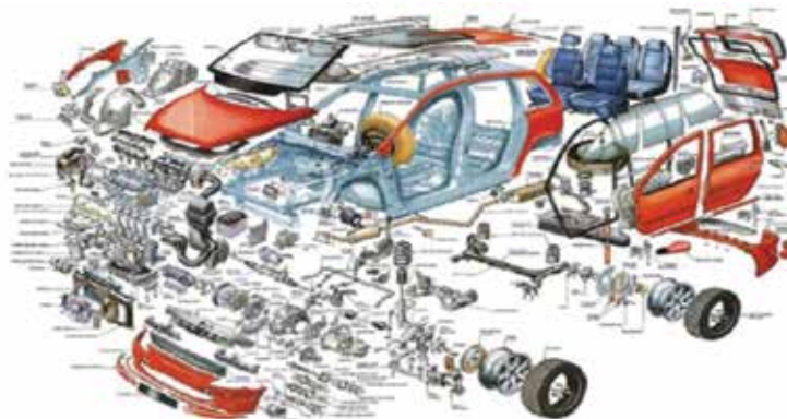
Figure 1. Exploded view of all car components.
