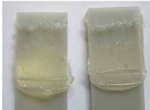
Figure 11. Failure surface of a SLJ test, overlap length 25 mm, adhesive thickness 1 mm.
