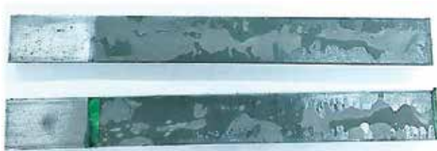
Figure 9. Failure surfaces for the DCB specimen.
