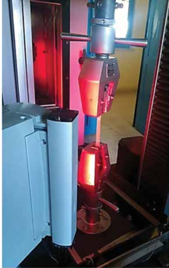
Figure 4. Tensile tester with video extensometer.
