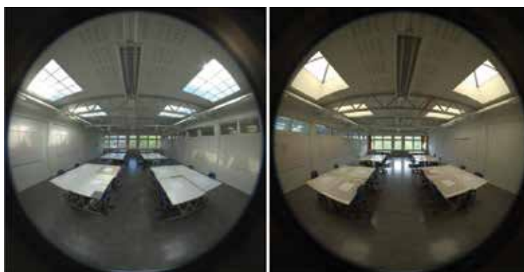
Figure 8. Fish eye HDR pictures of the studio under clear sky conditions, the new solution to the left, old one to the right.
