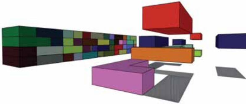
Figure 9. Modular architectural concept for multi-storey LSF buildings [4].
