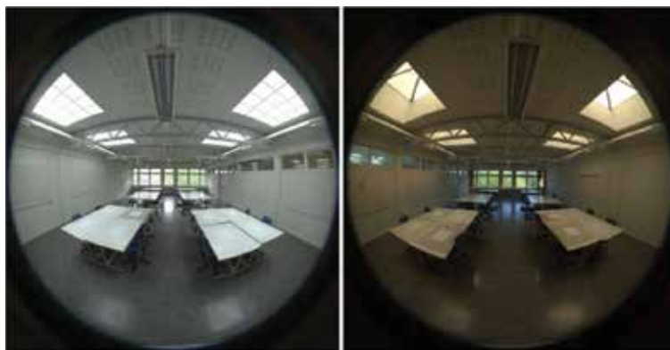
Figure 7. Fish eye HDR pictures of the studio under overcast sky conditions, the new solution to the left, old one to the right.
