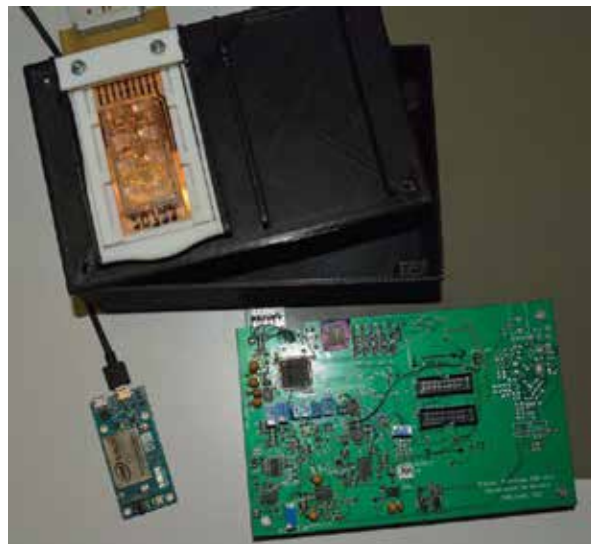
Figure 11. Photograph of the full measurement system including the electrodes for cell culture.
