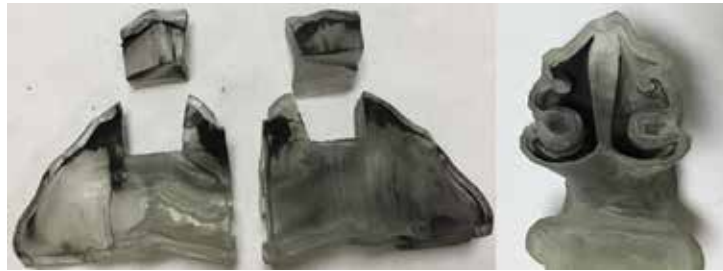
Figure 11. Deposition pattern in the right nasal passage and nasopharynx with the bi-directional delivery method. Appreciable deposition of particles was observed in the olfactory region. Because particles travel through the right and left passages in sequence, more particles were observed in the right passage than in the left passage.
