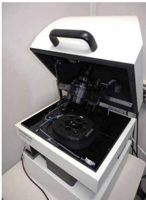
Figure 5. Bioluminescence microscope, LV200. A stage-top incubator with temperature and CO 2 gas controllers was added to the sample stage. The observation area was covered with a dark box.
