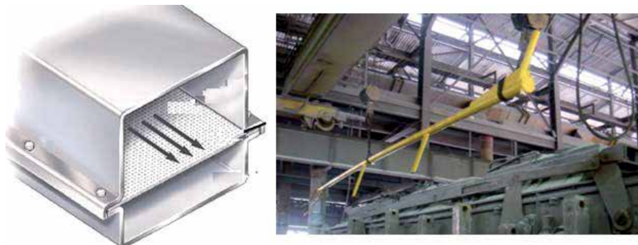
Fig. 18. The Albras aluminum smelter air fluidized conveyor and a conventional air slide in the left.
