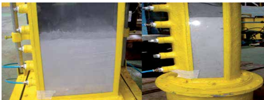
Fig. 19. Permeameters used at Albras laboratory to survey the minimum fluidization velocity of the powders used in the primary aluminum industry - source: Albras Alumínio Brasileiro SA.
