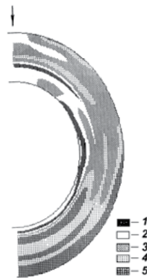
Fig. 10. Distribution of the relative heat transfer coefficient over the surface of type 2 fin ( h/d = 0.357 ) located in the frontal row of the bundle. Re = 2 \cdot 10^4 ; the free-stream direction is from the top down. a_i/a_{av} : 1) 1.94 to 1.66; 2) 1.66 to 1.24; 3) 1.24 to 0.83; 4) 0.83 to 0.41; 5) 0.41 to 0.11
