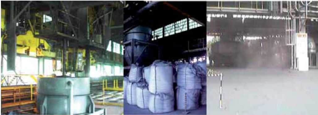
Fig. 16. Dust discharging at Albras bake furnace, implemented solution in the left side, in the center discharge of dust in big bags, free falling of dust in truck in the right - source: Albras Alumínio Brasileiro SA.
