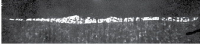
Fig. 8. Metallographic cross-section of laser irradiated steel sample.
