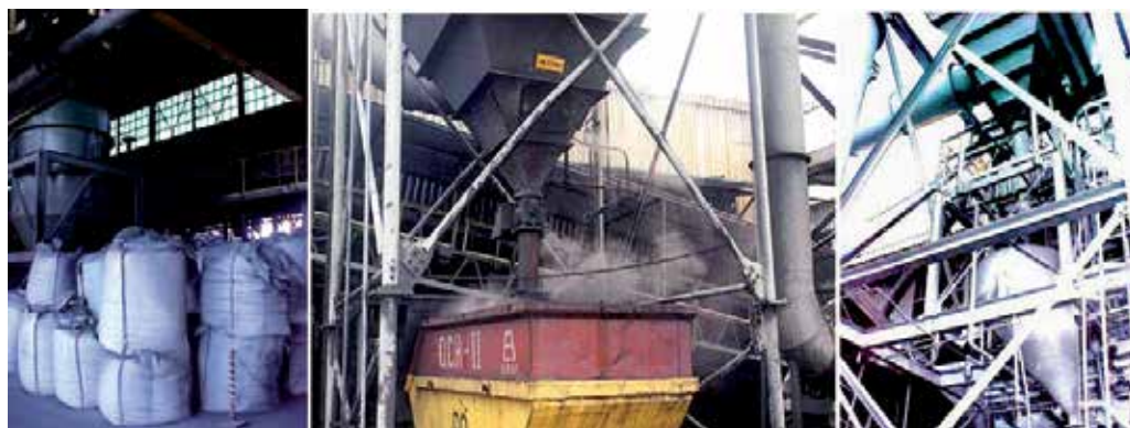
Fig. 15. Petro coke handling problem at Albras, in left bake furnace, in center and in the right bag house dust discharge at the rodding shop - source: Albras Alumínio Brasileiro SA.
