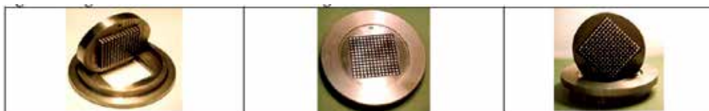
Fig. 3. A view of the extruder die for forming a monolithic carrier [42]
