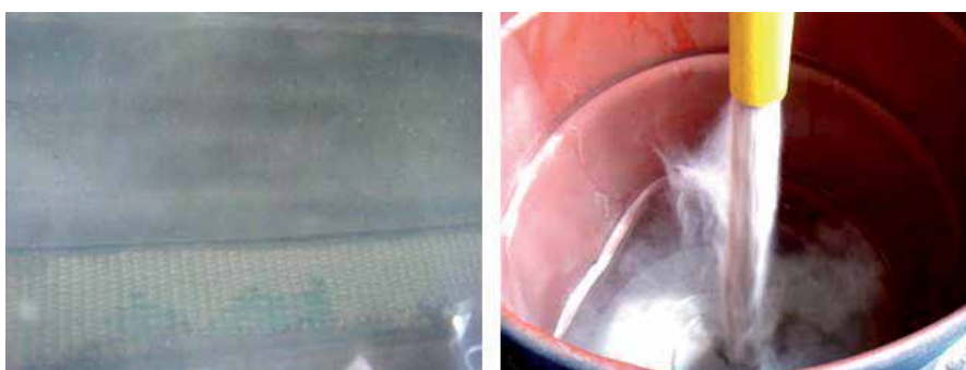
Fig. 22. Test rig to measure the mass solid flow rate of a, 9.3 m long 3 inches diameter air-fluidized conveyor at Albras aluminum smelter.
