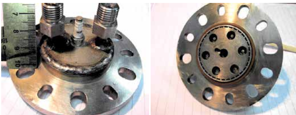
Fig. 12. Photography of mixing head.
