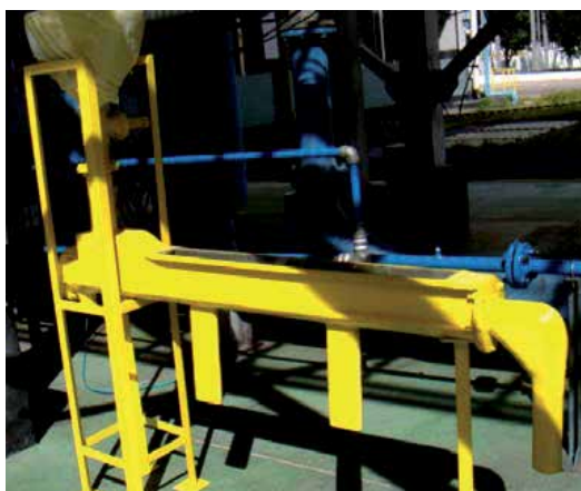
Fig. 20. Air-fluidized conveyor of 1.5 m long with three outlets.
