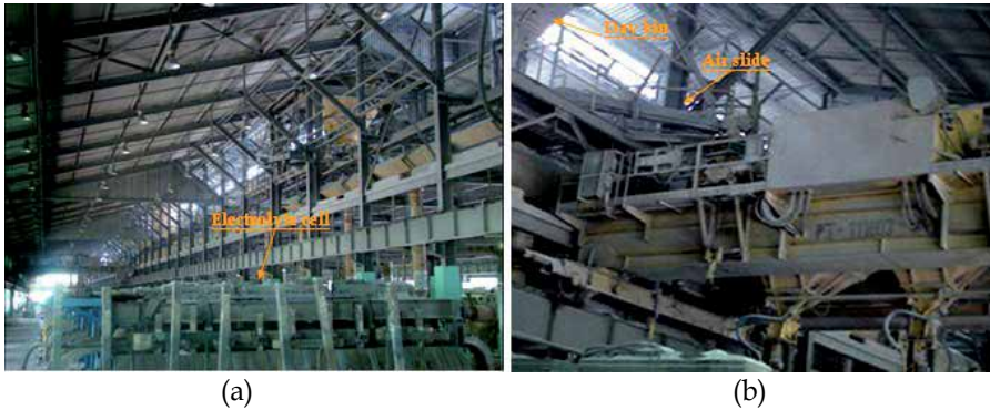
Fig. 2. a) Aluminum smelter pot room, b) Overhead crane being fed of alumina from a day bin by a standard air slide.
