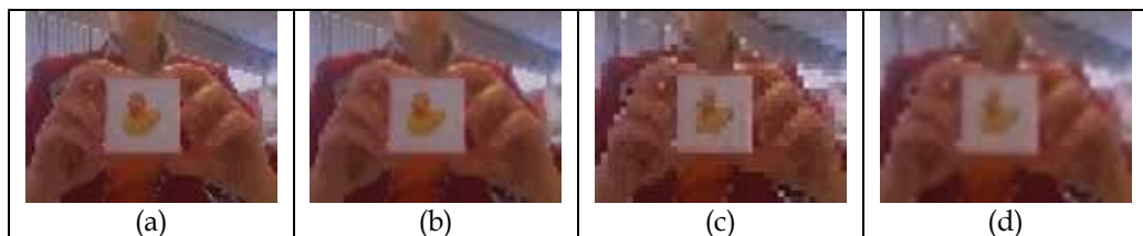
Fig. 8. Example frame of resolution (a) 80x60 and (c) 40x30 with cube sizes of 24x24 and 12x12 respectively. Figure (b) and (d) show these frames after they have been doubled in size using bilinear interpolation.
