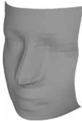
Fig. 7. The mean face template used for fine registration. The surface, composed of approximately 600 vertices, has been computed using a training set of manually normalized faces.
