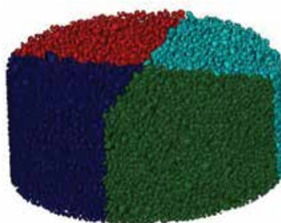
Figure 11. Modelled oedometer compression test separation into quarters [1].
