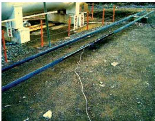
Fig. 4. Test to evaluate of equivalent thermal conductivity in the thermal insulated tubing using by pulsed heating carried at Yubari CO 2 -ECBMR test field (Oct. 10, 2006) (see Yasunami et al., 2010)
