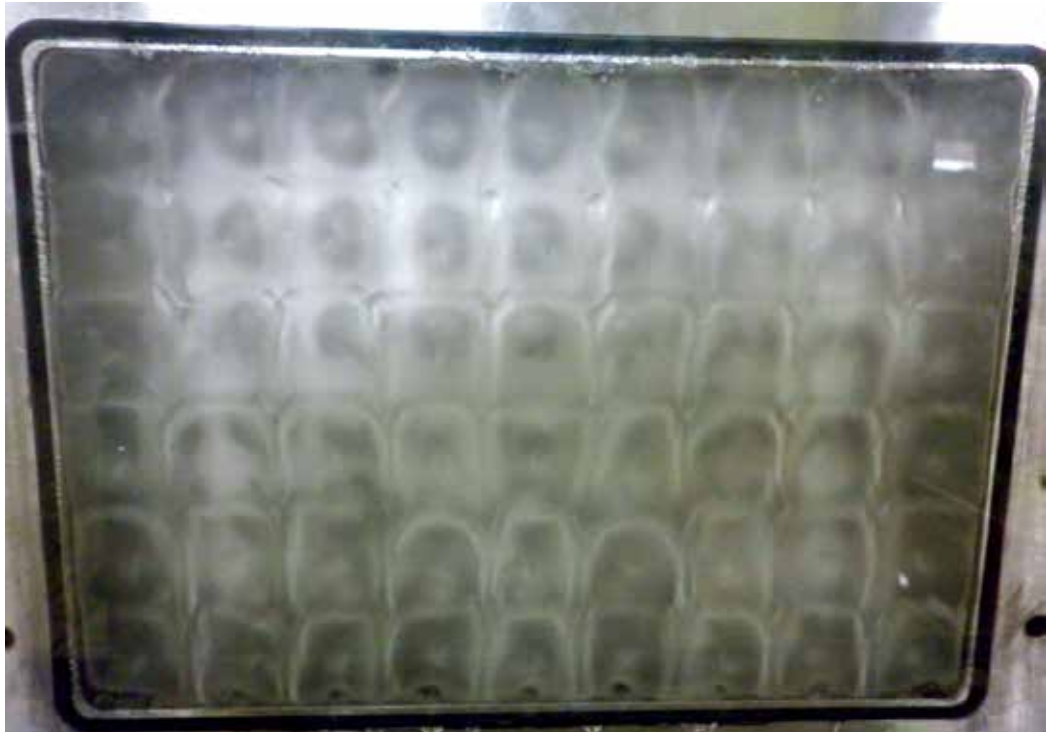
Fig. 20. A transparent surface impinged by a 54-nozzle spray
