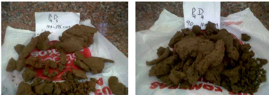
Figure 3. Clay soil samples were taken at depth >90 cm from the INIAP research station, Pichilingue, Ecuador ~containing ferrous and ferric minerals with the high values of specific surface area and water adsorption capacity (Final Report by Amer, 2014 [2] - SENESCYT, Prometeo Project, Ecuador).
