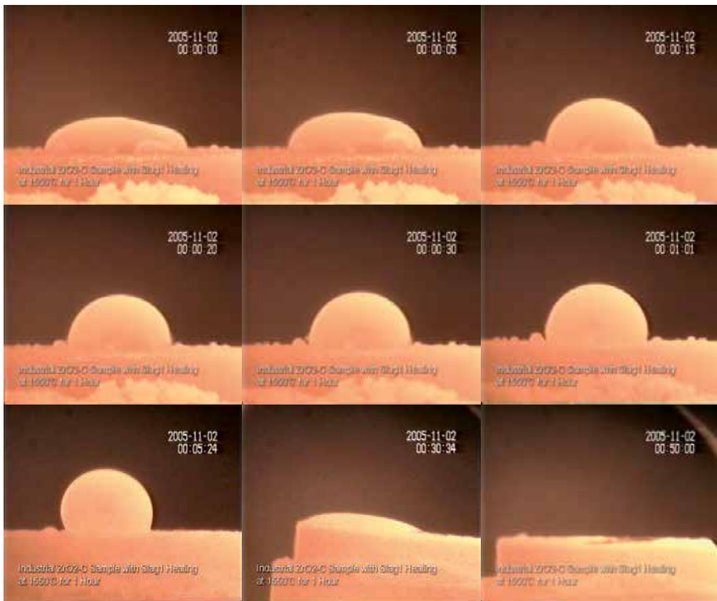
Figure 14. Industrial non-oxidized flat ZrO_2 -C samples with slag 1 (MnO 50%wt, SiO_2 25%wt, Al_2O_3 25%wt) heating at 1550°C for 1 hour
