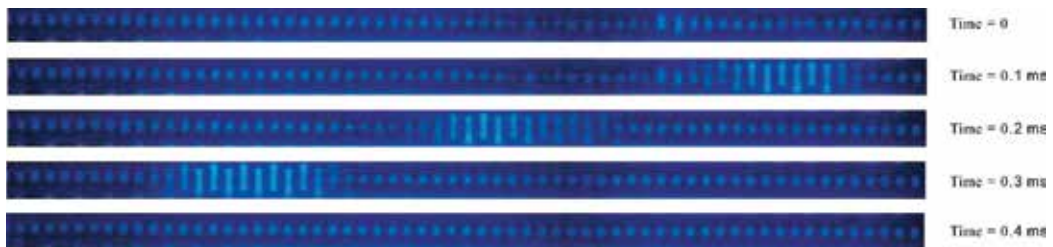
Fig. 10. Elongated slug bubble flow at G = 267 \text{ kg/m}^2\text{s} , q'' = 565.9 \text{ kW/m}^2 , and x = 0.14
