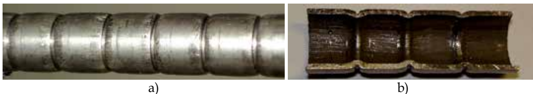
Fig. 9. Photos of a discretely rough tube: a) outside view; b) sectional view
