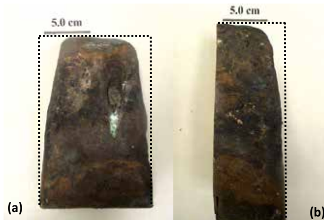
Fig. 1. Hot end of water cooled copper finger after being removed from a flash furnace. (a) Front view, (b) lateral view. The dotted lines represent the original dimensions of the cooler.
