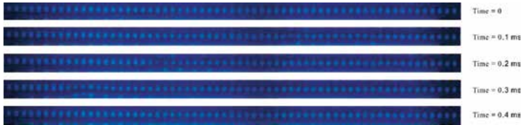
Fig. 11. Annular flow at G = 169 \text{ kg/m}^2\text{s} , q'' = 422.3 \text{ kW/m}^2 , and x = 0.27
