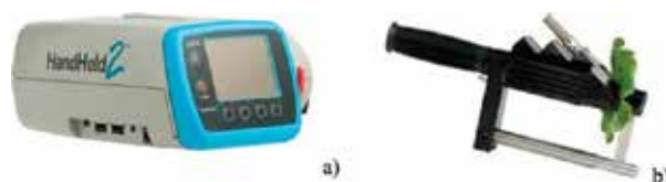
Figure 5. (a) ASD Hand Held 2 spectrophotometer (b) plant probe + leaf clip.
