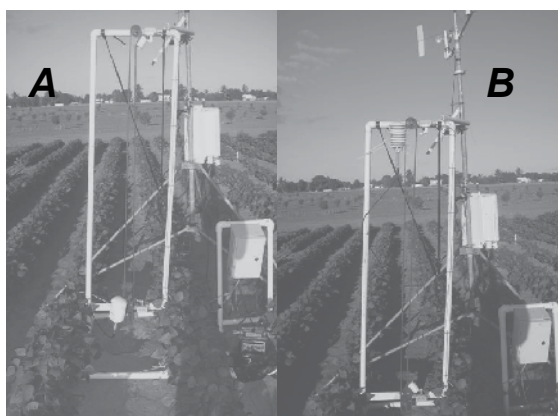
Fig. 2. Automated elevator device developed for moving the Temp/RH sensor between the two vertical positions. A. Temp/RH sensor in down position and B. Temp/RH sensor in up position. Measuring over common bean ( Phaseolus vulgaris L.). (These data's were obtained under the project sponsored by NOAA-CREST (NA17AE1625), NASA-EPSCoR (NCC5-595), USDA-TSTAR-100, USDA Hatch Project H-402, and University of Puerto Rico Experiment Station)
