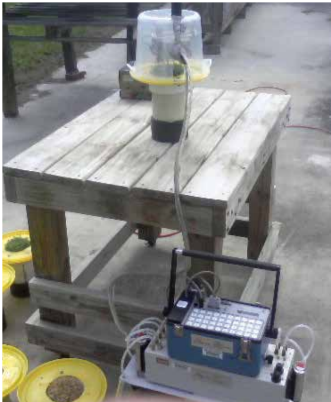
Fig. 9. Portable chamber system for measuring canopy gas exchange
