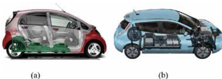
Figure 2. Schematics of two well-known pure EVs, showing the position of the main power devices: batteries, inverter, and electrical machine. (a) Rear-wheel drive and (b) front-wheel drive. Original images extracted from [3, 4] and modified by the authors.
