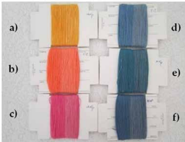
Figure 3. Dyeings with 0.5% selected dyes: (a) Levafix Amber CA, (b) Remazol Orange RR, (c) Remazol Red RB 133%, (d) Remazol Navy GG 133%, (e) Remazol Black B 133%, (f) Remazol Blue RR (for each shade: untreated yarn on the left side, UV faded on the right side).
