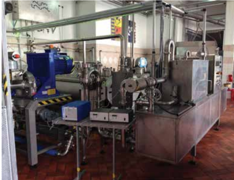
Figure 2. The sono-exchanger system and the three drivers, which provide the periodic signals (Colletorto, Italy, Aloia farm).
