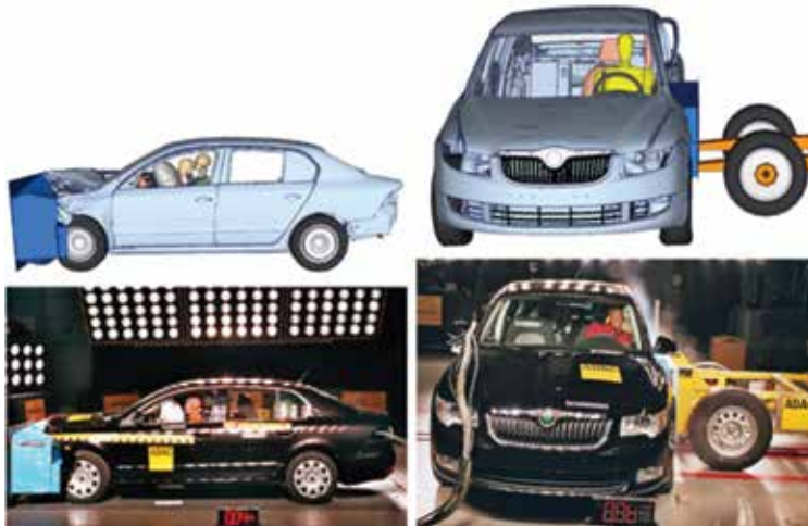
Figure 7. The vehicle crash test and simulation.
