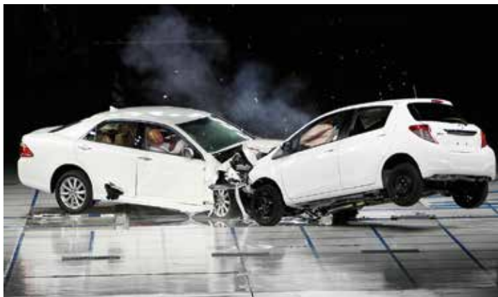
Figure 6. Vehicle-to-vehicle impact test of Toyota Motor Company.
