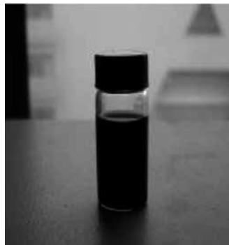
Figure 32. Photograph of the Cu@Ni nanoparticles stored in PAO6 after one month.
