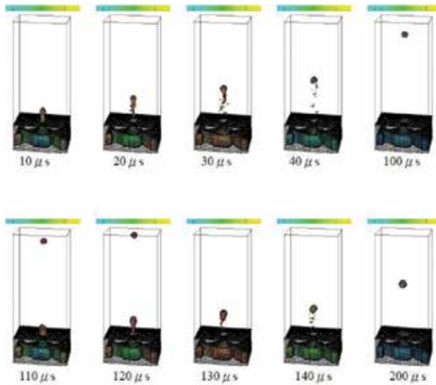
Figure 15. Numerical simulation of DNA in the nozzle diameter 30\ \mu\text{m} and 50\ \mu\text{m} thickness tapered dual channel injection chamber to 10\ \text{kHz} operating frequency, three-dimensional side view, in 10, 20, 30, 40, 100, 110, 120, 130, injection of the case 140 and 200\ \mu\text{s} .
