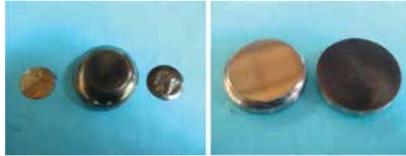
Figure A1. The photos of the ingot with cut off upper and lower “caps” before (left) and after (right) cutting into two halves which served as billets for the fabrication of mirror samples.
