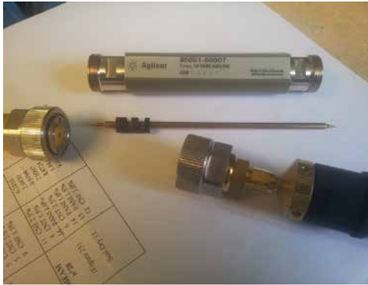
Figure 2. Coaxial airline 50 Ω probe used for the dielectric characterization of nanocomposite materials and for the measurement of EM reflection and transmission properties of layered materials.
