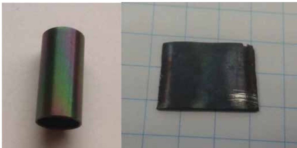
Figure 8. Left: A sample of PCD-coated zirconium fuel cladding; right: a lengthwise cut of a sample of PCD-coated zirconium fuel cladding, which after being exposed to water vapour at 400°C for 3 days was completely straightened. The PCD layer has withstood even this strain without compromising its integrity. The scratch in the right lower corner (right) was made using a diamond point pen.
