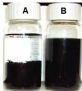
Figure 1. Nanofluid prepared by dispersing MWCNTs in deionized water (A) shows that MWNTs deposited at the bottom of the container and (B) shows that MWNTs maintain good dispersion: From Ref. [43].
