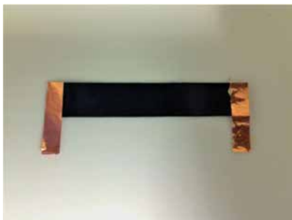
Figure 2. CNT sheet assembled between two polyethylene terephthalate (PET) tapes with Cu electrodes attached at both ends to form a CNT heater.
