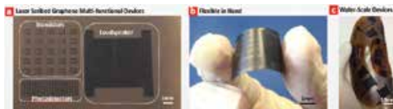
Figure 25. Wafer-scale graphene devices integration. (a) Multifunctional graphene devices containing transistors, photodetectors and loudspeakers. (b) Flexible graphene devices. (c) Wafer-scale graphene devices. Reprinted by permission from Macmillan Publishers Ltd: Scientific Reports (4:3598), copyright (2014) [16].
