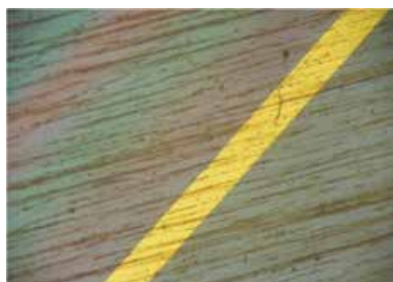
Figure 12. Microscopy image of 0.016 wt.% SWNT-COOH, 0.016 wt.% \text{Fe}_2\text{O}_3 in DI water. At 8 min, the internal reference is 30 \mu\text{m} . From Ref. [70].
