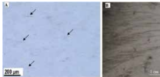
Figure 13. Alignment of CNFs in epoxy. (A) Optical microscopy images for 0.002 wt.% CNFs, 0.002 wt.% \text{Fe}_2\text{O}_3 , and 0.02 wt.% NaDDBS in epoxy after 48 h. (B) Digital camera image of 0.02 wt.% CNFs, 0.02 wt.% \text{Fe}_2\text{O}_3 , and 0.2 wt.% NaDDBS in epoxy after 2 h. Magnetic field ( H = 1.2 \text{ kG} ) was applied. From Ref. [30].
