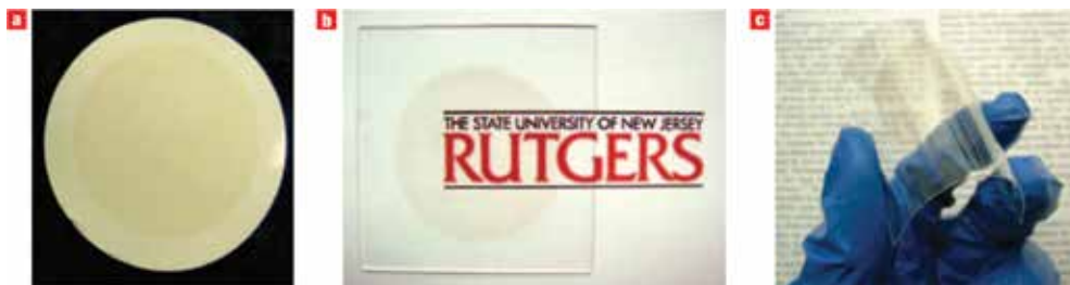
Figure 1. GO film obtained via the vacuum filtration method. (a) GO film on filter paper. (b) GO film on glass. (c) GO film on polyethylene terephthalate (PET). Reprinted by permission from Macmillan Publishers Ltd: Nature Nanotechnology (3:270), copyright (2008).[8].
