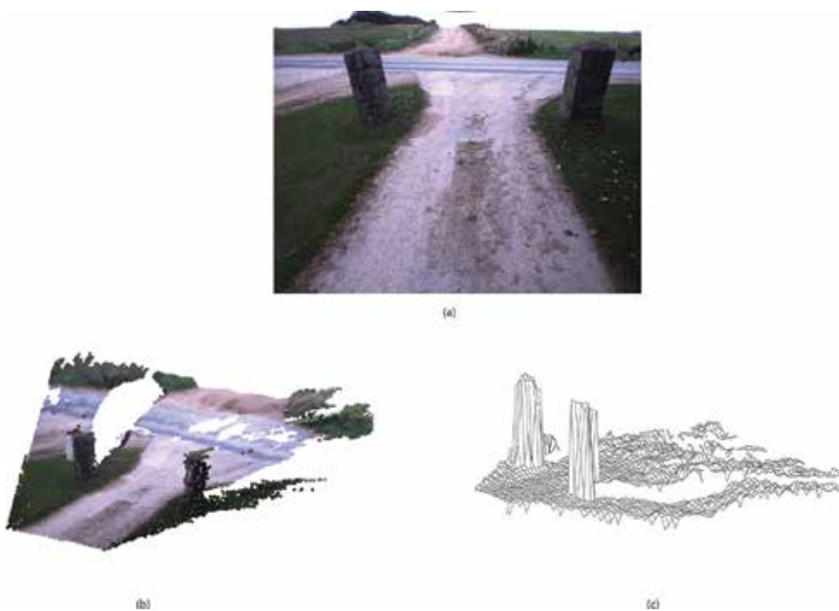
Figure 2. Example of two different space representations in which (b) is a point cloud representation, whereas (c) is the relative DEM, both geometrically describing the scene in the camera image (a).
