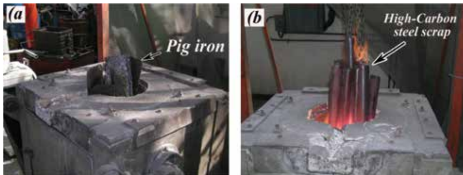
Figure 8. Induction furnace charged to produce cast iron, (a) when using pig iron as raw material and (b) when using steel scrap.
