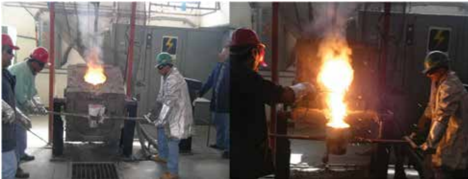
Figure 9. Pouring the liquid iron into the preheated ladle in the ductile iron making.
