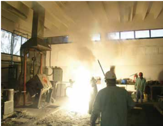
Figure 10. Nodulising ductile iron with magnesium, note the intensity of the reaction when magnesium is added into the liquid metal.
