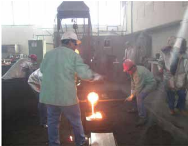
Figure 11. Pouring the liquid iron into sand moulds.
